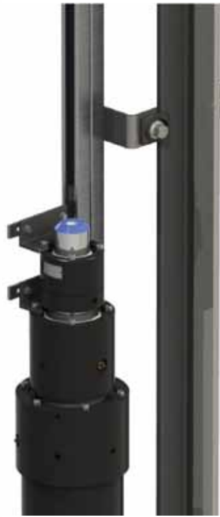
Figure 3: A three-stage jack
