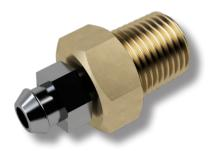
The 1/8" NPT Jack Bleeder Assembly (A879) is compact and easily installed. This bleeder is rated at 1500 psi. The barbed bleeder screw enables use of a 1/4" I.D. soft plastic or rubber tubing to direct oil into a container while bleeding the jack.
