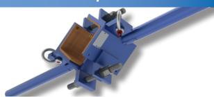
**Piston Clamp/Wrenches (PCW)** are designed to safely lift, hold, and tighten pistons during construction. The welded steel construction with replaceable tension pads and tensioning bolts for applying equal pressure around a piston ensures higher gripping force than wooden clamps. The maximum rated load for the Piston Clamp/Wrench is 1,950 lbs.
