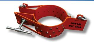
**PVC Lifting Clamps (PVCC)** are designed to lift and hold flush joint PVC pipe safely. Constructed of formed and welded 1/4" steel plate for light weight and easy handling, these clamps are equipped with two holding tabs and shackles for lifting. A tee bolt tensioner is used to apply pressure around PVC pipe with cupped set screws for gripping. The maximum rated load for the PVC Lifting Clamp is 3,000 lbs.
