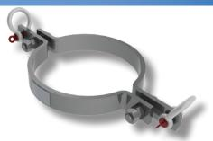
**Cylinder Lifting Clamps (CLC)** are designed to lift and hold hydraulic jack cylinders safely during construction. Constructed of formed steel bar for light weight and easy handling. These clamps are equipped with shackles for lifting and tensioning bolts for applying pressure around cylinder pipe.
