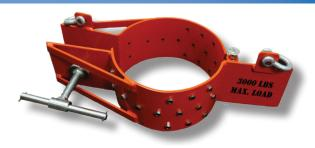
**PVC Lifting Clamps (PVCC)** are designed to lift and hold flush joint PVC pipe safely. Constructed of formed and welded 1/4" steel plate for light weight and easy handling, these clamps are equipped with two holding tabs and shackles for lifting. A tee bolt tensioner is used to apply pressure around PVC pipe with cupped set screws for gripping. The maximum rated load for the PVC Lifting Clamp is 3,000 lbs.
