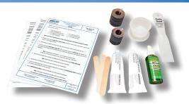
This **Piston Repair Kit (PRK-01)** is designed to repair damaged pistons with deep scratches or pits that cause excessive weeping of oil through the seals. The two part metal filled epoxy is ideal for filling in deep scratches and pits that are too deep to be removed with just light sanding. Using this kit, once properly applied, can prolong a damaged piston and seal life.
