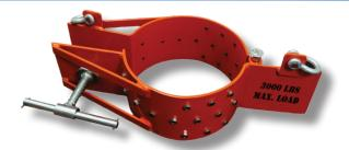
**PVC Lifting Clamps (PVCC)** are designed to lift and hold flush joint PVC pipe safely. Constructed of formed and welded 1/4" steel plate for light weight and easy handling, these clamps are equipped with two holding tabs and shackles for lifting. A tee bolt tensioner is used to apply pressure around PVC pipe with cupped set screws for gripping. The maximum rated load for the PVC Lifting Clamp is 3,000 lbs.
