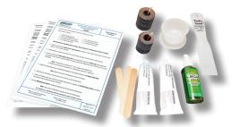
This **Piston Repair Kit (PRK-01)** is designed to repair damaged pistons with deep scratches or pits that cause excessive weeping of oil through the seals. The two part metal filled epoxy is ideal for filling in deep scratches and pits that are too deep to be removed with just light sanding. Using this kit, once properly applied, can prolong a damaged piston and seal life.
