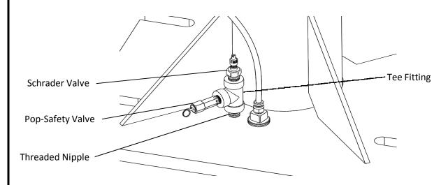
4. Apply thread sealant to all threads. Thread nipple into Tee Fitting and then tighten the threaded Nipple with Tee Fitting into the 1/4" port of the Pit Plate. Then tighten the Schrader Valve to the Tee Fitting and lastly tighten Pop-Safety Valve to Tee Fitting as shown. Make sure all fittings are pressure tight.
