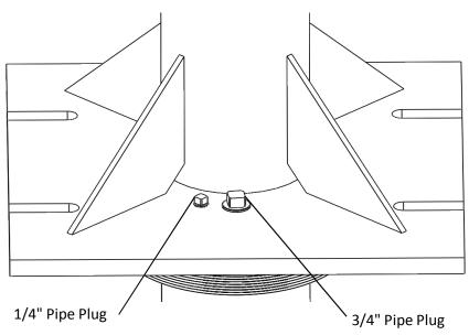
1. Remove the 3/4" pipe plug and the 1/4" pipe plug from the base plate.
