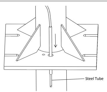
2. Push end of Evacuation Kit with the steel tube through the 3/4" hole until it hits the bottom of the PVC Liner.
