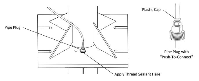
3. Apply thread sealant to the 3/4" Pipe Plug and then tighten. To adjust slack in tube, hold down plastic cap on brass "Push-To-Connect", pull/push tube through top of pipe plug as needed to reach the bottom.
